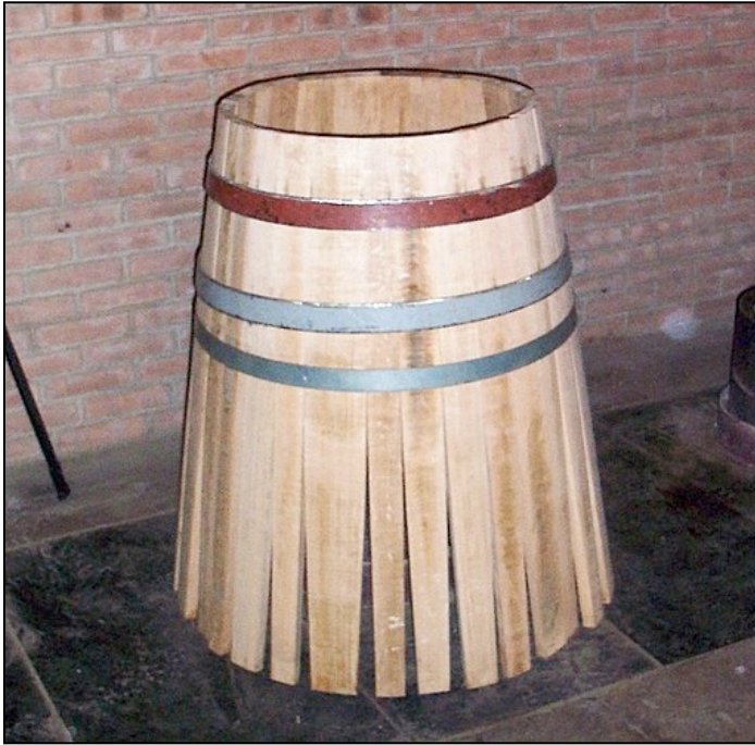
A partially assembled wine barrel showing initial arrangement of the staves. The oak staves here are much thicker than those of the lime barrels.
