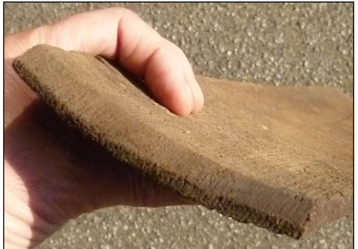
Close-up of the top of a stave, showing curve and beveled end.
