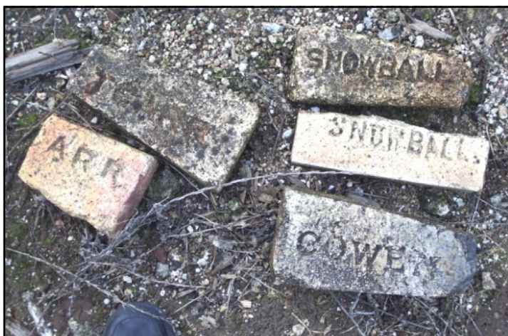
These loose firebricks photographed near the kilns in 2006 show all three brands: two SNOWBALL bricks (upper right), one COWEN (lower right), and two T. CARR (left, one incomplete). The bricks are about 9 inches long.
